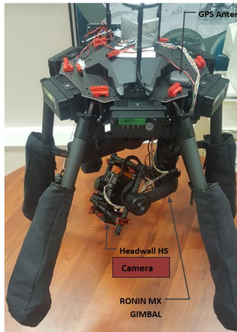
Figure 3. SERCE multi-rotor air vehicle and gimbal + Headwall HS camera position (Aselsan, 2017)
