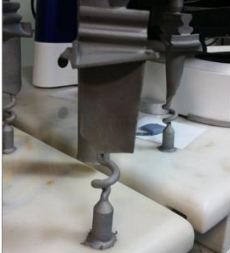
Figure 23. First superalloy turbine blades cast in Türkiye.
