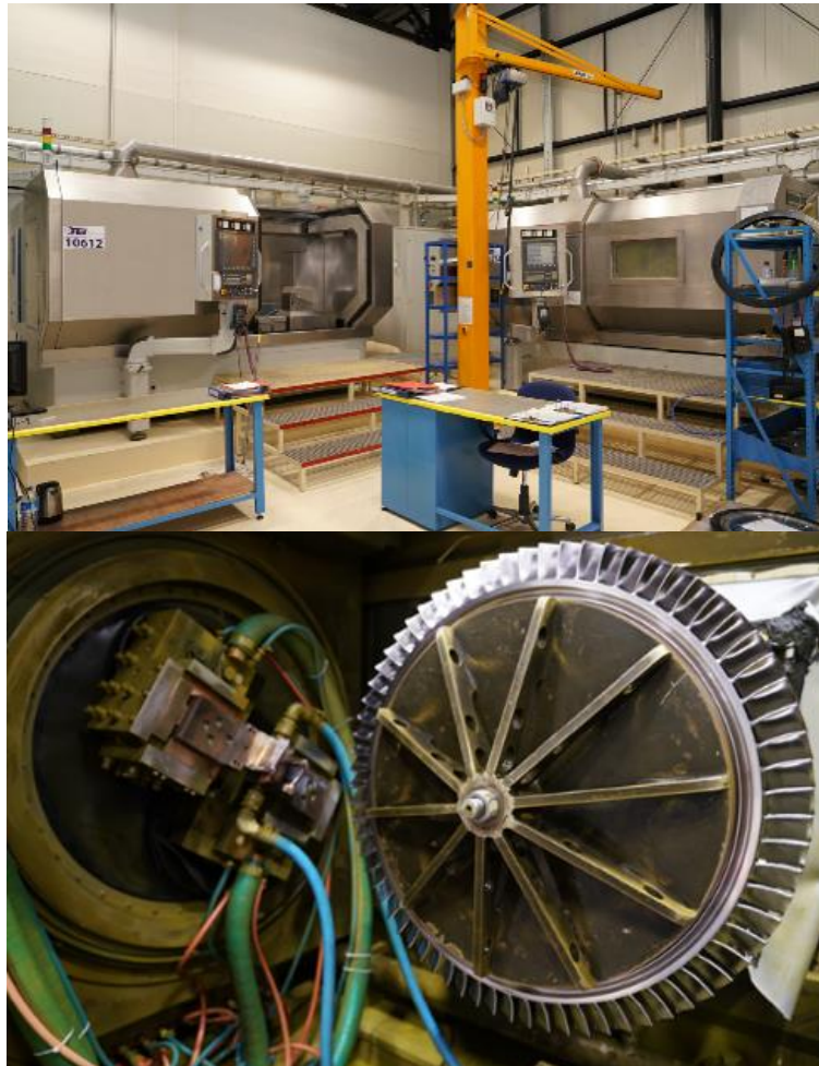
Figure 37. 6-Axis Electro-Chemical Processing Technology Providing High Material Removal Capability for Super Alloy Materials
