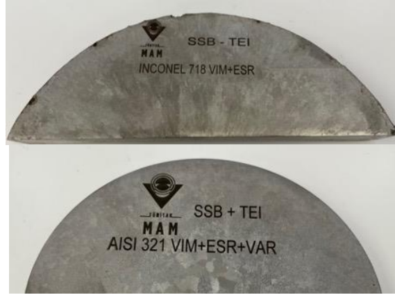
Figure 26. First aerospace-quality IN718 Nickel Superalloy and AISI 321 stainless steel produced in Türkiye
