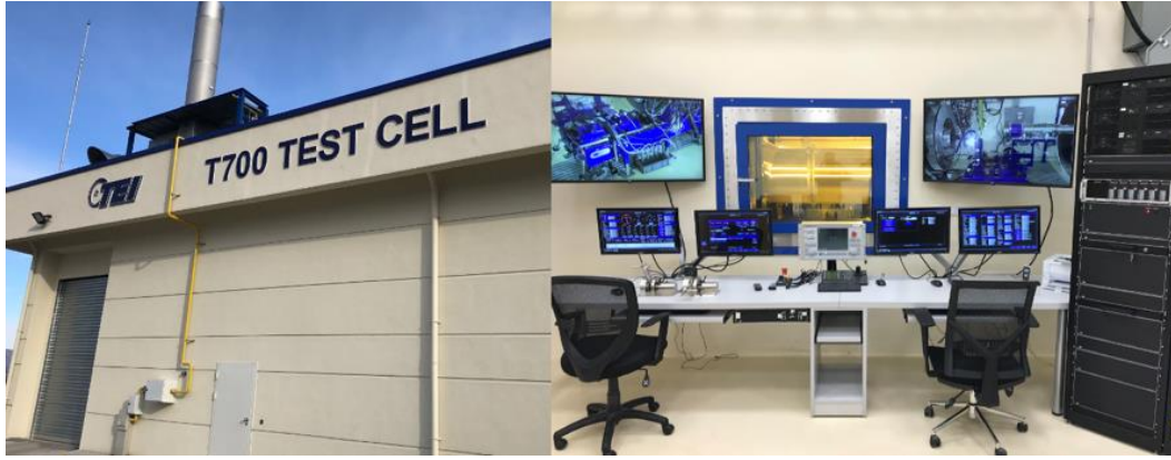
Figure 20. Engine test bench established for test and qualification of domestic production T700-TEI-701D Engines at TEI Eskişehir facilities
