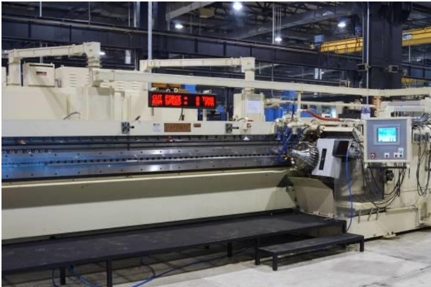
Figure 31. Turbine disc broach opening process
