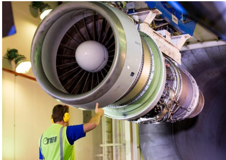
Figure 19. 100.000 lbf thrust capacity Turbofan/Turbojet Engine Test Bench at TEI Eskişehir facilities
