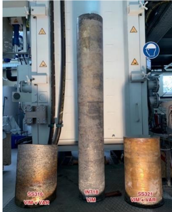
Figure 27. The first aerospace-quality IN718 Nickel Superalloy, AISI 316L and AISI 321 stainless steel produced at TÜBİTAK MAM laboratories in Türkiye, in the form of billets as they come out of the furnace
