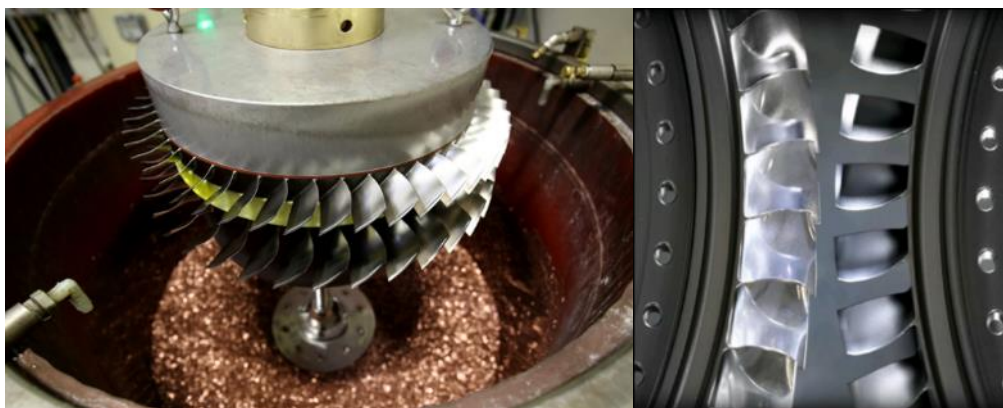
Figure 40. Engine compressor performance is increased by reducing the roughness level of Blisk blades with ultrapolish process
