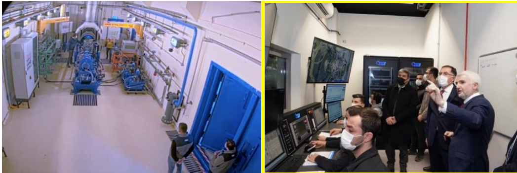
Figure 15. First national engine test bench designed, developed, built and commissioned for testing and qualification of TEI-TS1400 Turboshaft Engine by TEI engineers and technicians
