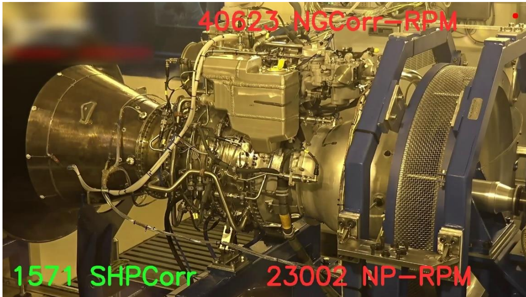
Figure 16. TEI-TS1400 Turboshaft Engine being tested in the national engine bench developed by TEI, together with accessory systems such as national gearbox, oil tank and pump
