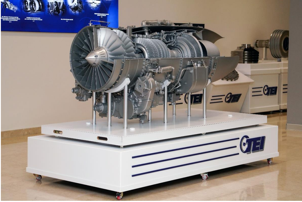
Figure 17. Türkiye's first turbofan engine, TEI-TF6000 technology demonstrator
