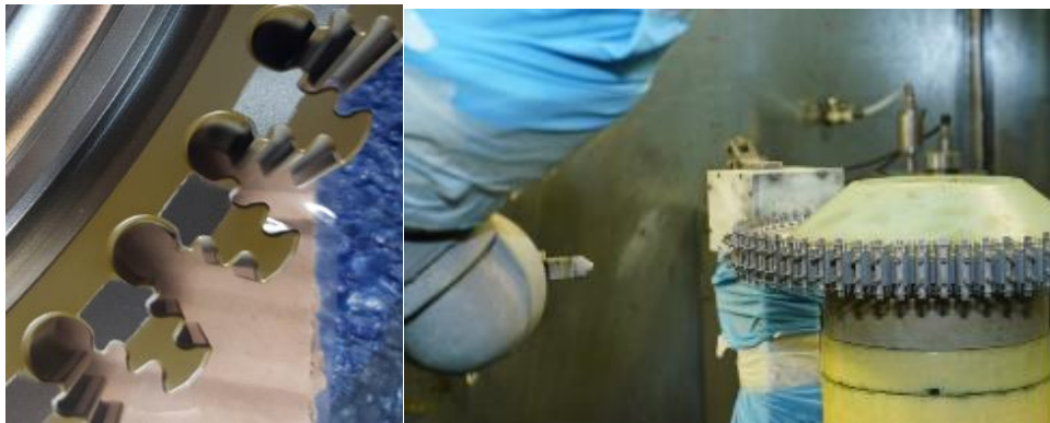
Figure 39. TEI applies anti-corrosion coating technology on turbine disks to increase thermal shock resistance of the materials under high temperatures
